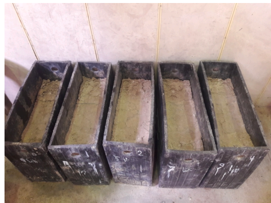
Fig. 13. Ballast box samples after testing (specimens from left to right correspond to 0, 0.09, 0.15, 0.21 and 0.27 lit/m 3 of RRP235 Special).
